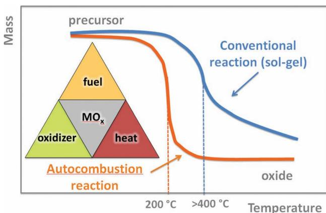
Figure 27. Schematic comparison of the decomposition profile of a combustion precursor and conventional sol-gel reaction (adapted from [340]).
