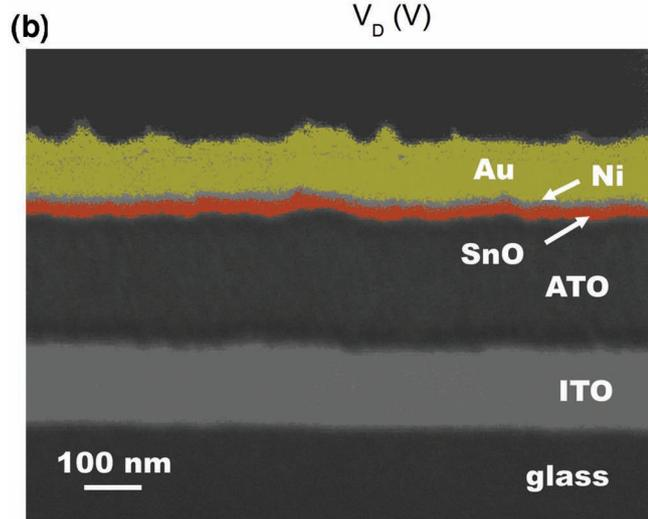
**Figure 47.** a) Typical output characteristic of SnO p-channel TFT (gate voltage is varied from 0 to -50 V in -10 V steps); b) TFT SEM cross-section where it is clearly shown all the constituent layers.
