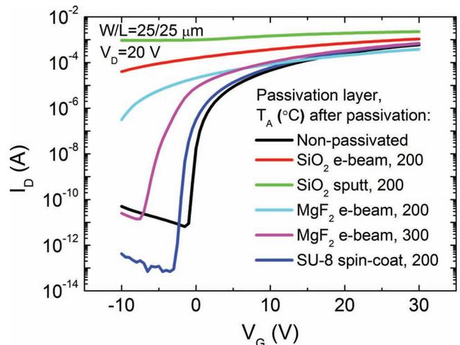
**Figure 16.** Transfer characteristics obtained for GIZO TFTs with different passivation layers (adapted from [277]).
