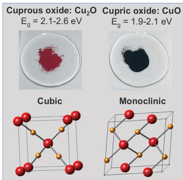
**Figure 31.** Copper (I) oxide or cuprous oxide is one of the principal oxides of copper. The compound can appear yellow or red, depending on the size of the particles.  $\text{Cu}_2\text{O}$  crystallizes in a cubic structure. Copper (II) oxide or cupric oxide belongs to the monoclinic crystal system. It is a black solid with an ionic structure.
