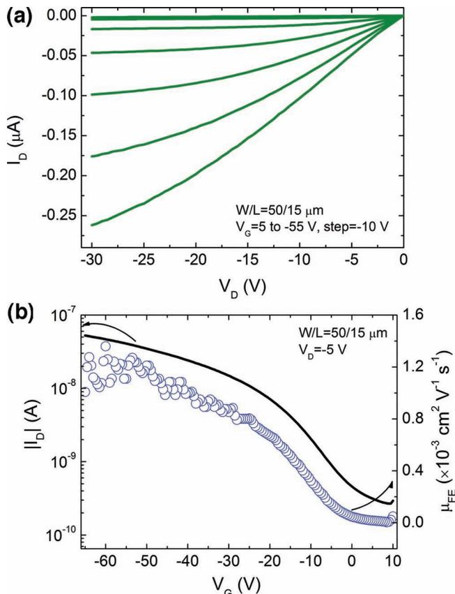
**Figure 36.** a) Output characteristics ( $I_D$ - $V_D$ ); b) Transfer characteristics ( $|I_D$ - $V_G$ ) at  $V_D = -5$  V (left axis) and  $\mu_{\text{FE}}$  as a function of  $V_G$  (right axis), for a typical  $\text{Cu}_2\text{O}$  TFT produced at room temperature and annealed in air at 200 °C. The inset shows the structure of the bottom gate TFT (adapted from [431]).
