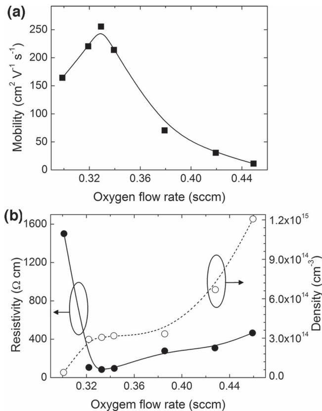
**Figure 33.** Mobility (a) and resistivity and hole density (b) of  $\text{Cu}_2\text{O}$  thin films with LTB- $\text{Cu}_2\text{O}$  as a function of oxygen flow rates.<sup>[419]</sup>
