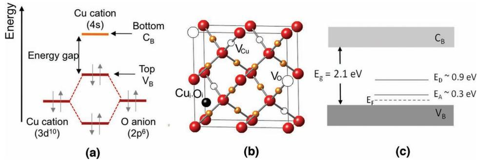
**Figure 32.** a) Chemical bond between an oxide ion and a cation that has a closed-shell electronic configuration; b) representation of the more important defects in  $\text{Cu}_2\text{O}$ ; c) a simple electronic model proposed by Brattain, with a compensated semiconductor with one acceptor level at 0.3 eV and a deep donor level at 0.9 eV from  $V_B$  (adapted from [431]).
