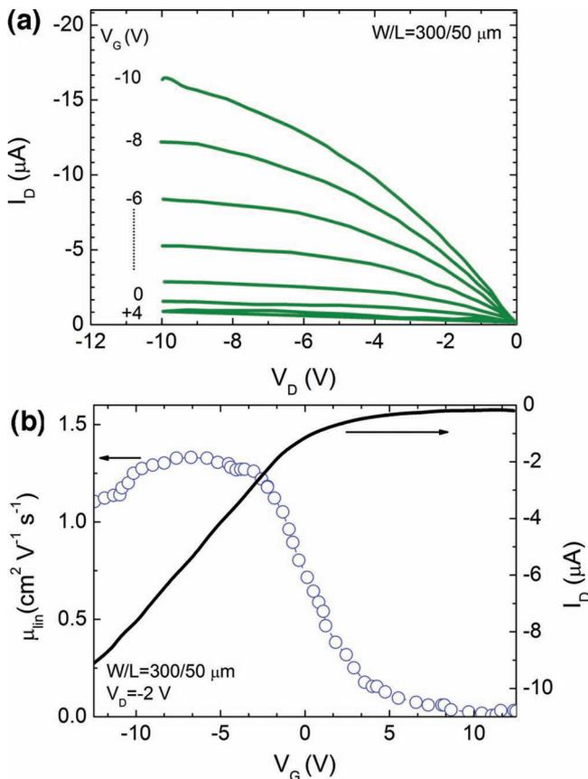
**Figure 44.** a) Output characteristics and b) field effect mobility in the linear region ( $\mu_{\text{lin}}$ ) as a function of  $V_G$  (adapted from [472]).
