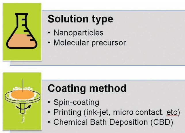
**Figure 23.** Solution type and coating methods used for solution-processed TFTs.
