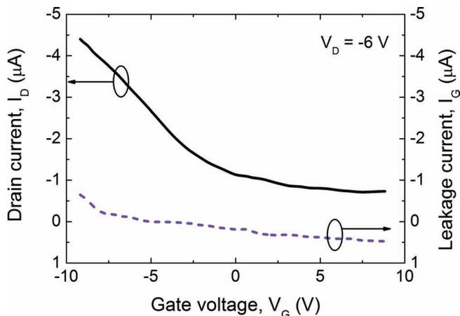
**Figure 35.** Transfer characteristic  $I_D$ - $V_G$  of  $\text{Cu}_2\text{O}$  channel TFT at  $V_D = -6$  V (adapted from [420]).
