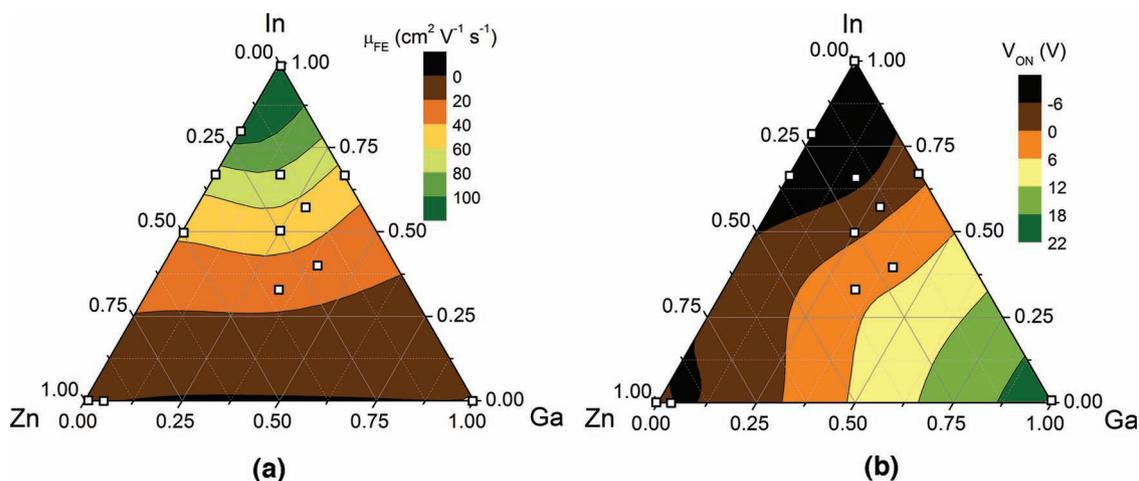
**Figure 13.** a)  $\mu_{FE}$  and b)  $V_{ON}$  obtained for TFTs with different oxide semiconductor compositions, in the gallium-indium-zinc oxide system. Devices annealed at 150 °C, with %O<sub>2</sub> = 0.4%.
