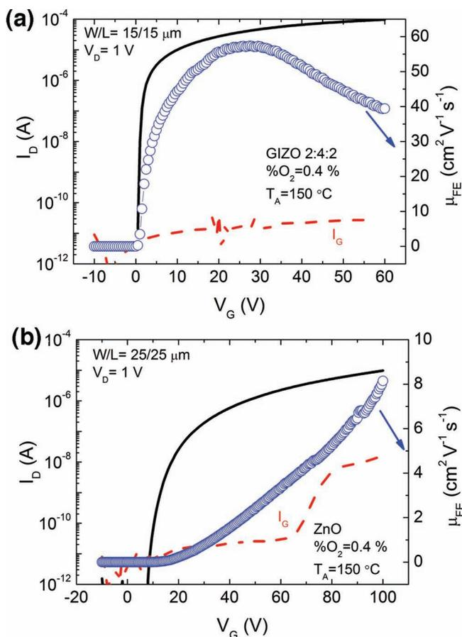
**Figure 14.** Transfer characteristics and  $\mu_{FE}$ - $V_G$  plots measured for high  $V_G$  for TFTs annealed at 150 °C, based on a) GIZO 2:4:2 and b) ZnO.
