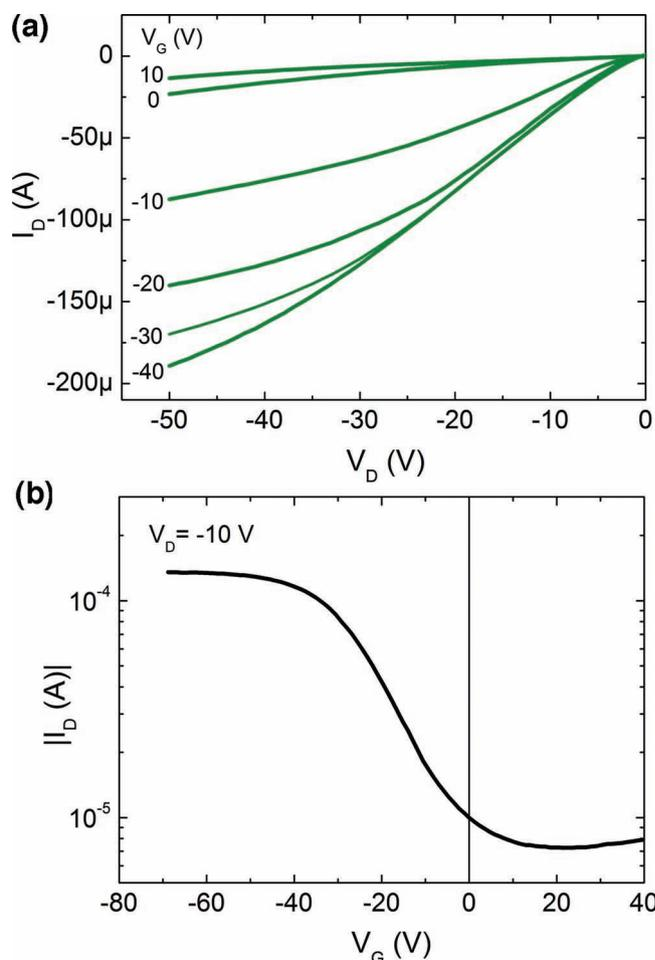
**Figure 48.** a) Output characteristics ( $I_D$ - $V_D$ ) and; b) Transfer characteristics ( $|I_D$ - $V_G$ ), for a SnO<sub>x</sub> p-type paper transistor produced at room temperature and annealed in air at 160 °C.
