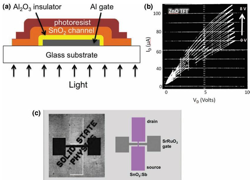
**Figure 4.** Initial TFTs employing oxide semiconductors as channel layers: a) Schematic of the  $\text{SnO}_2$  TFT reported by Klasens and Koelmans in 1964, to show a new self-aligned lift-off process;<sup>[30]</sup> b) Source-drain voltage-current characteristic of a single crystal ZnO FET, c) Picture and layout of the ferroelectric Sb: $\text{SnO}_2$  TFT proposed by Prins et al. in 1996.<sup>[31]</sup>
