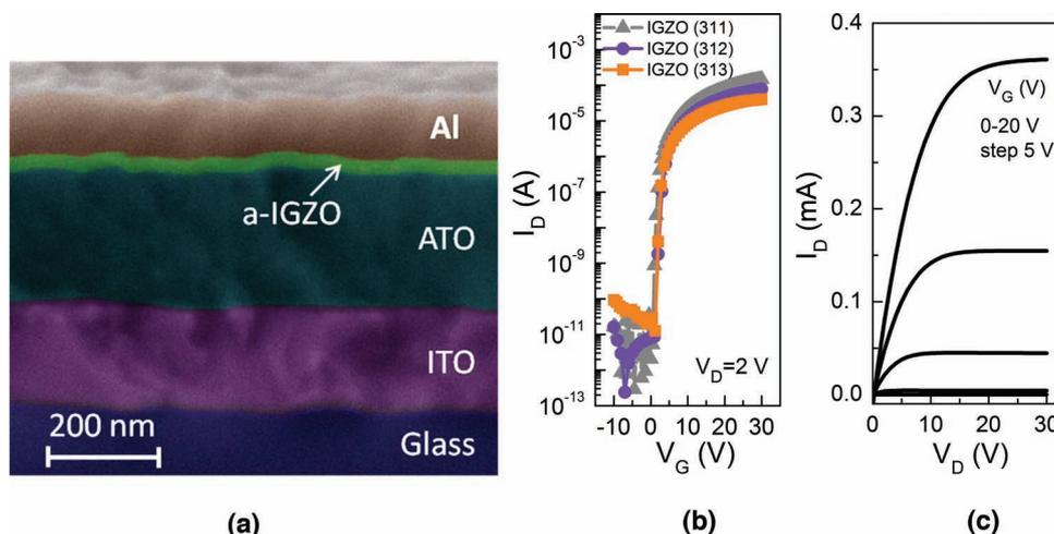
Figure 25. a) Cross sectional SEM image of GIZO (311) TFT; b) Transfer and c) Output characteristics of GIZO TFTs with different compositions (adapted from [337]).
