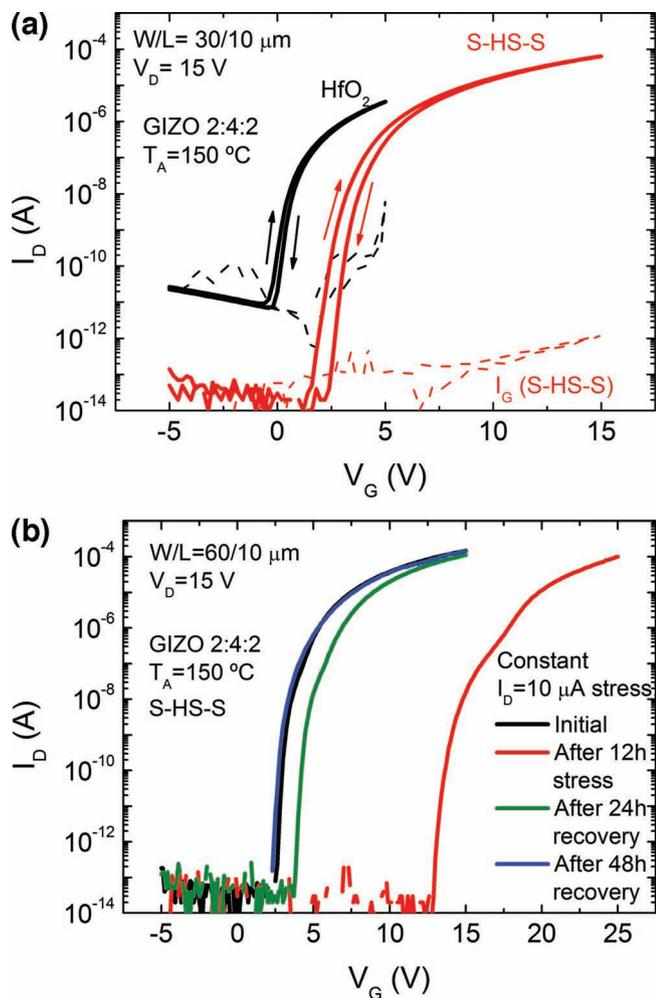
**Figure 20.** Electrical properties obtained for GIZO TFTs with Hf-based dielectrics: a) transfer characteristics for HfO<sub>2</sub> and S-HS-S devices; b) transfer characteristics evolution for S-HS-S TFTs during constant I<sub>D</sub> stress measurements. Devices annealed at 150 °C.
