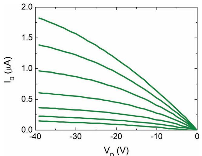
**Figure 34.**  $I_D$ - $V_D$  curves for a p-channel TFT employing  $\text{CuZnO}_x$  as the channel layer and a thermal  $\text{SiO}_2$ -silicon substrate bottom gate. The channel layer is subjected to a post-deposition furnace anneal in air at 800 °C in air. For this device,  $V_{\text{ON}} \approx -60$  V,  $\mu_{\text{INC}} \approx 0.01$   $\text{cm}^2 \text{V}^{-1} \text{s}^{-1}$ , and  $W/L = 5$  (adapted from [30]).
