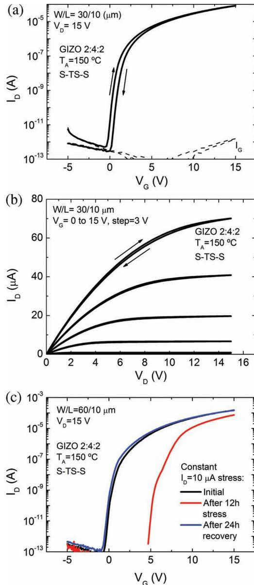
**Figure 19.** Electrical properties obtained for GIZO TFTs with S-TS-S dielectric: a) transfer characteristics; b) output characteristics; c) transfer characteristics evolution during constant  $I_D$  stress measurements. Devices annealed at  $150 \text{ } ^\circ\text{C}$ .
