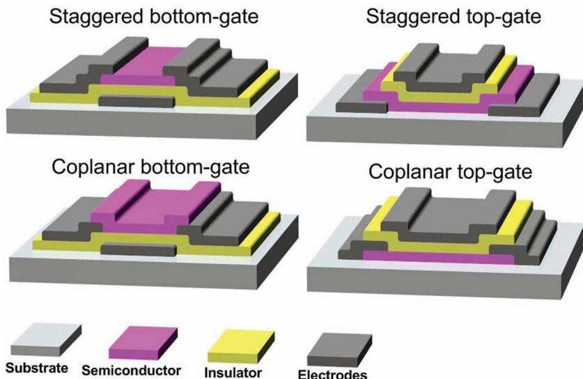
**Figure 7.** Schematics showing some of the most conventional TFT structures, according to the position of the gate electrode and to the distribution of the electrodes relatively to the semiconductor.
