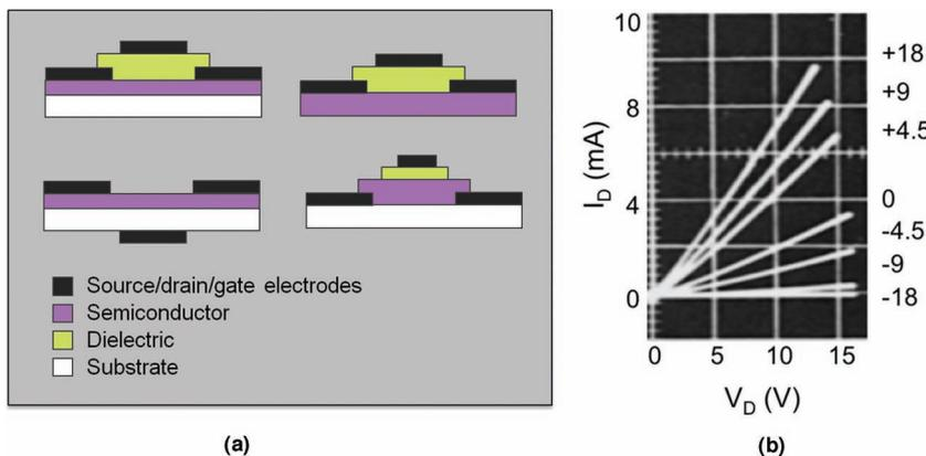
**Figure 22.** a) Examples of the tested insulated gate field effect devices used by Sihvonen et al. and b) Output characteristic of a device using an inorganic ink-dielectric layer (adapted from [322]).
