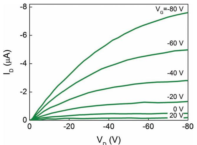
**Figure 45.** Drain current as a function of drain voltage at various gate voltages for the top-contact  $\text{SnO}_2$  TFTs (adapted from [473]).
