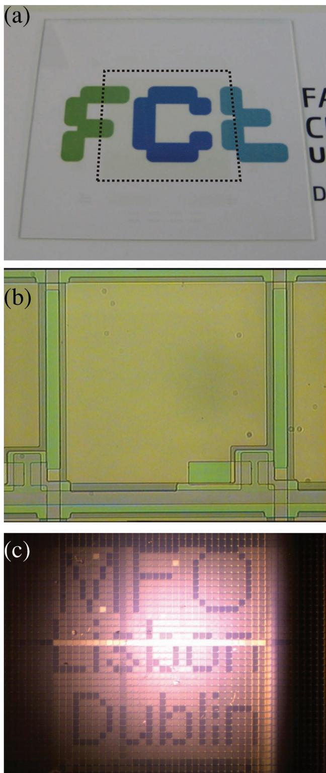
**Figure 51.** AM backplane with GIZO TFTs produced at CENIMAT for a LCD display: a) photograph of a transparent AM on glass; b) microscopy image of pixel area ( $350 \times 350 \mu\text{m}$ ); c) prototype after integration with LCD front plane.<sup>[303]</sup>
