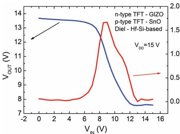
**Figure 56.** VTC and gain for a transparent CMOS inverter with n-type GIZO and p-type SnO TFTs fabricated at CENIMAT/13N.
