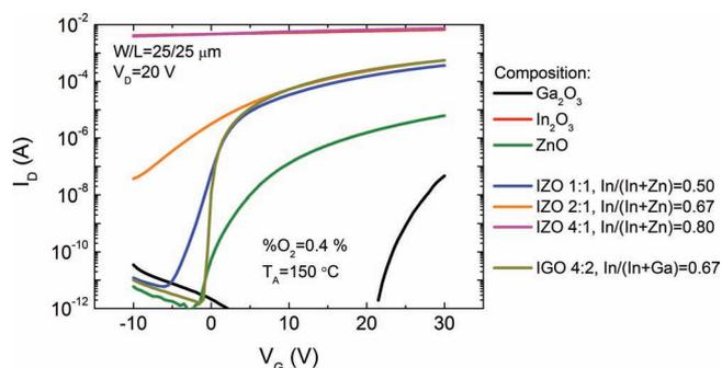
**Figure 11.** Effect of oxide semiconductor target composition on the transfer characteristics of TFTs annealed at 150 °C: binary and ternary compounds.
