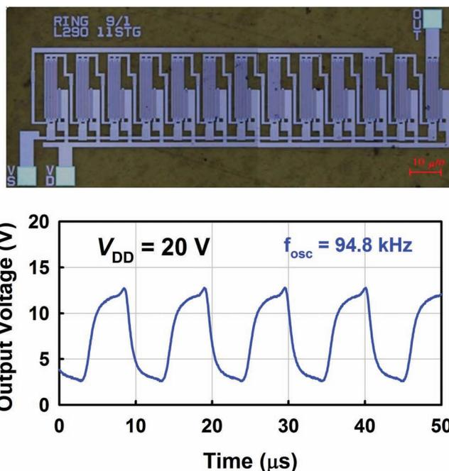
**Figure 54.** a) Optical image of an eleven-stage RO, and b) output characteristics of the fabricated ring oscillator on plastic substrates (adapted from [220]).
