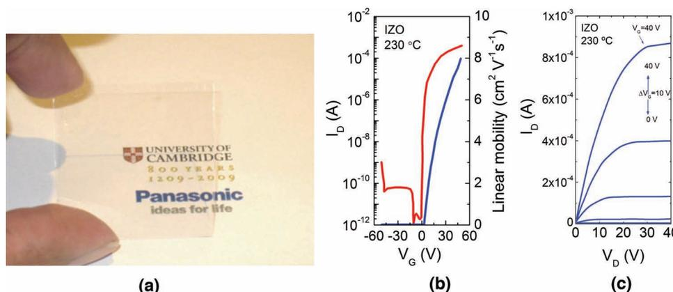
Figure 26. a) Photograph of a transparent, hydrolysed films; b) Transfer and c) Output characteristics of IZO TFTs produced under hydrolysed conditions (adapted from [338]).
