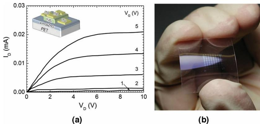
**Figure 5.** a)  $I_D$ ,  $V_D$  characteristics of a flexible substrate with transparent a-GIZO TFTs; Photograph of the flexible TFT sheet bent at  $R = 30$  mm presented by Nomura et al. in 2004 (adapted from [10]).
