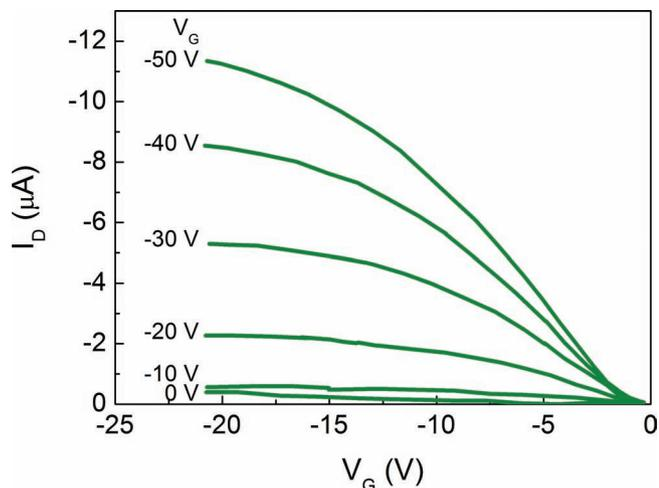
**Figure 46.** The characteristics of drain-source current ( $I_D$ ) vs drain-source ( $V_D$ ) for the TFT with the SnO channel annealed at 400 °C (adapted from [476]).
