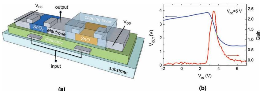
**Figure 58.** Schematic of a conceptual CMOS inverter using n-type SnO<sub>2</sub> and p-type SnO TFTs (adapted from [477]); b) VTC for an ambipolar SnO CMOS inverter (adapted from [483]).
