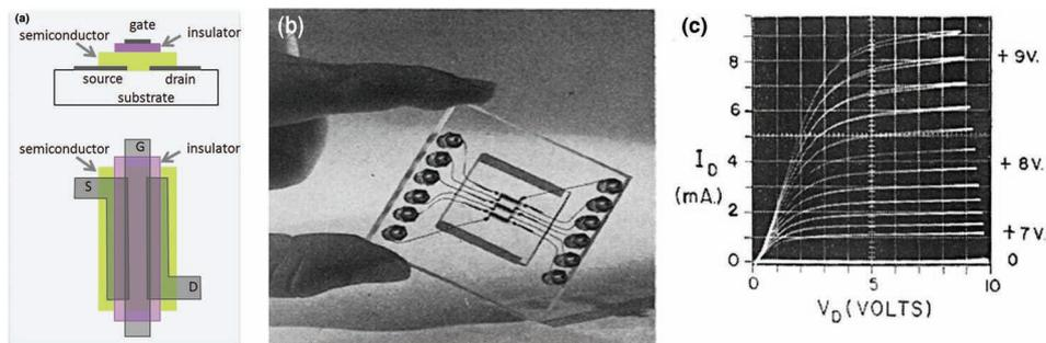
**Figure 3.** a) Cross-sectional view and top view, b) A 1-in square glass plate (mounted on a lucite block) upon which 3 TFTs have been deposited and c) Output characteristics of CdS TFTs reported by Weimer (adapted from [27]).
