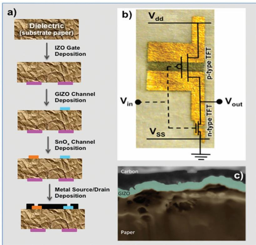
**Figure 59.** a) Cross sectional schematic of fabrication sequence of the paper-CMOS showing all layers that constitute the final device and how they are interconnect as well as image of the real device; b) Image of the real paper-CMOS and c) SEM cross section of the n-type paper TFT.
