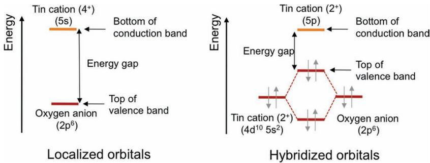
**Figure 43.** Comparison between the band structure of  $\text{SnO}_2$  and  $\text{SnO}$ . In the case of  $\text{SnO}$  the top of the valence band consist of hybridized orbital of O  $2p$  and Sn  $5s$ .
