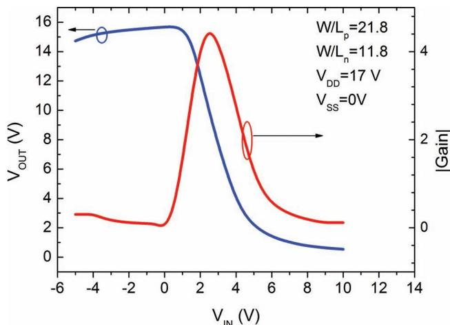
**Figure 60.** Voltage transfer characteristic of the paper CMOS under a  $V_{DD} = 17$  Volts (right scale) and the CMOS gain, exceeding 4.
