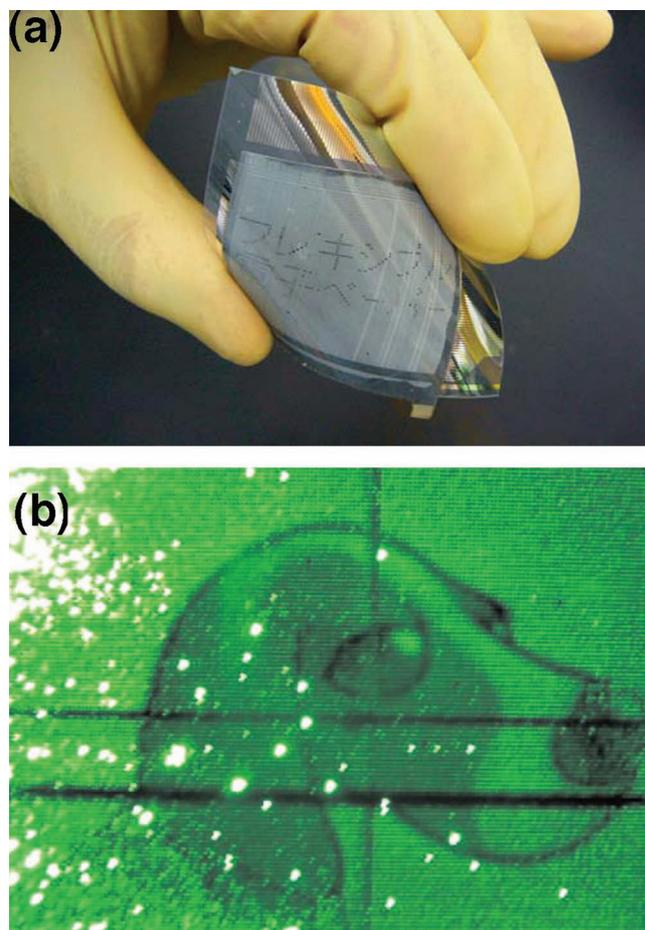
**Figure 52.** Prototypes of displays with oxide TFT backplanes: a) flexible electrophoretic display;<sup>[487]</sup> b) OLED display driven by solution-processed IZO TFTs.<sup>[490]</sup>
