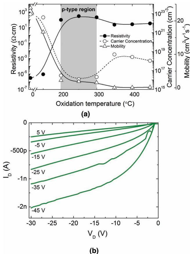
**Figure 39.** a) Dependence of the resistivity of  $\text{Cu}_x\text{O}$  films as a function of oxidation temperature; b) p-type TFT with  $\text{Cu}_2\text{O}$  channel layer oxidized in air at 200 °C.
