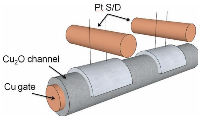
**Figure 41.** Schematic of  $\text{Cu}_2\text{O}$  transistor on Cu wire. Inner core Cu and outer shell  $\text{Cu}_2\text{O}$  film are used for the gate and channel, respectively. Source and drain pads are made by Pt by thermal evaporation, and the source and drain interconnection is made by cross-woven Cu wire, adapted from [457].
