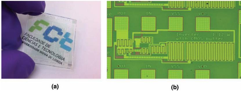
**Figure 55.** a) Transparent CMOS inverters on glass; b) optical microscopy image of an oxide CMOS inverter.
