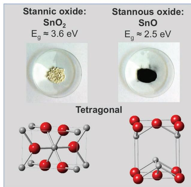
**Figure 42.** Unit cell of the crystal structure of  $\text{SnO}_2$  and  $\text{SnO}$ .
