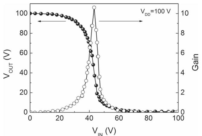
**Figure 57.** VTC and gain for a CMOS inverter with p-type  $\text{SnO}_x$  and n-type  $\text{In}_2\text{O}_3$  TFTs (adapted from [474]).
