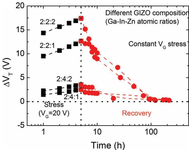
**Figure 15.**  $\Delta V_T$  obtained on gate-bias stress measurements during 5 h, for oxide TFTs with different GIZO compositions, annealed at 150 °C.
