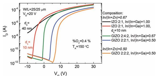
**Figure 12.** Effect of oxide semiconductor target composition on the transfer characteristics of TFTs annealed at 150 °C: ternary and quaternary compounds. The effect of decreasing  $d_s$  from 40 to 10 nm for IZO 2:1 is also shown.
