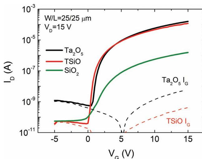
**Figure 18.** Transfer characteristics of GIZO TFTs using sputtered  $SiO_2$ ,  $Ta_2O_5$  and co-sputtered TSiO dielectrics. Devices annealed at  $150^\circ C$  (adapted from [303]).
