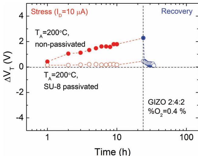
**Figure 17.**  $\Delta V_T$  vs stress/recovery time obtained from constant  $I_D$  stress measurements of GIZO TFTs with and without SU-8 passivation,  $\%O_2 = 0.4\%$  and  $T_A = 200^\circ C$  (adapted from [312]).
