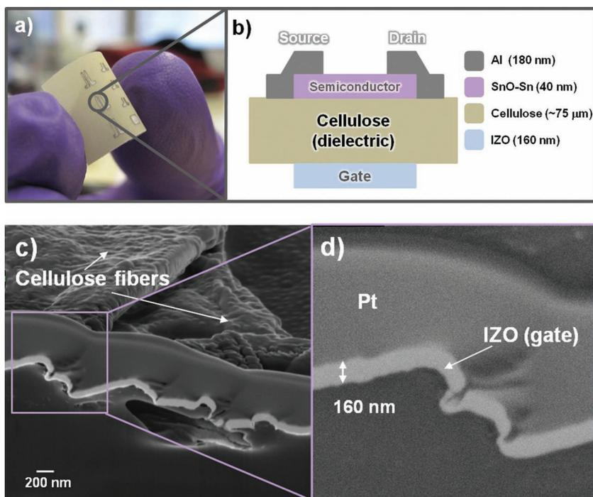
**Figure 49.** a) shows an optical photograph of a p-type paper transistor; b) architecture of the paper transistor; c) scanning electron microscopy cross section image of the gate electrode (IZO<sup>[481,482]</sup>) and d) with a higher magnification to see the detail of the good step coverage of the oxide semiconductor over the cellulose fibers.
