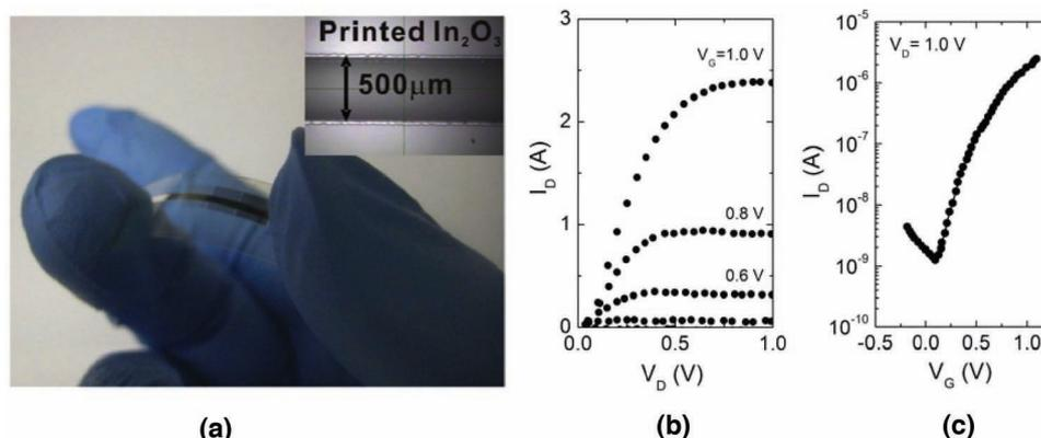
**Figure 28.** a) Optical photograph of a flexible combustion-processed  $\text{In}_2\text{O}_3$  device on Acrylite (30 nm Al gate electrode/41 nm  $\alpha$ -alumina dielectric, the inset shows an optical image of an ink-jet printed Al/41 nm  $\alpha$ -alumina dielectric; b) output characteristics and c) transfer characteristics (adapted from [339]).
