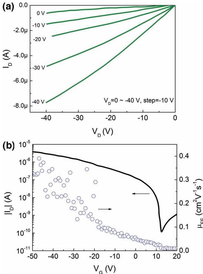
**Figure 37.** a) Drain current-drain voltage  $I_D$ - $V_D$  characteristics of a thin-film transistor based on an active layer of the postannealed CuO at 300 °C. The gate voltage,  $V_G$  varied from 0 to 40 V in steps of 10 V and b) the source-to-drain current,  $I_D$  as a function of gate voltage,  $V_G$  at a fixed drain voltage of -10 V measured in air (adapted from [450]).
