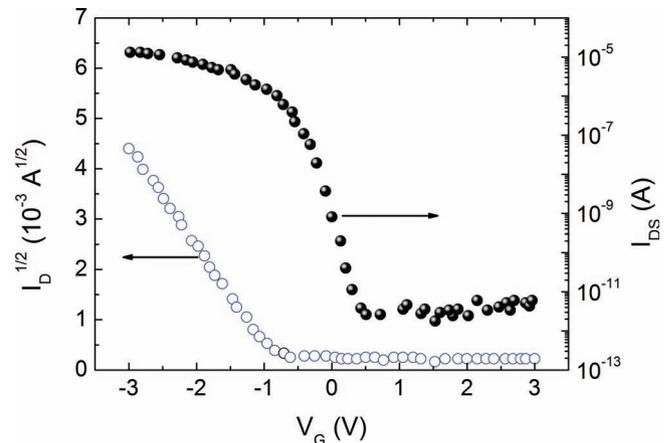
**Figure 38.** Transfer characteristics of p-channel  $\text{Cu}_2\text{O}$  TFTs with  $W/L = 500/20 \mu\text{m}$ .  $V_G$  was swept from -3 to 3 V at  $V_D = 3 \text{ V}$  (adapted from [451]).
