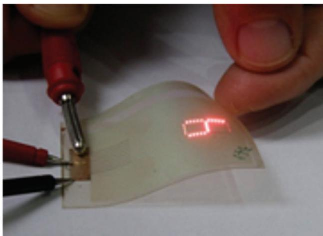
**Figure 50.** Transparent PM chipLED display using IZO electrodes.
