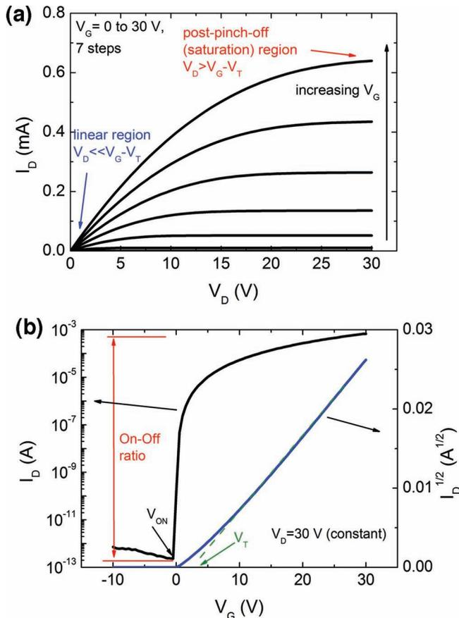
**Figure 9.** Typical a) output and b) transfer characteristics of a n-type oxide TFT.
