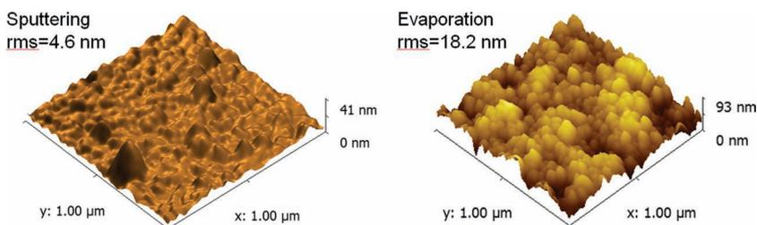
**Figure 40.** Surface roughness measured by AFM for a) a  $\text{Cu}_2\text{O}$  thin film grown by rf magnetron sputtering and b) a  $\text{Cu}_2\text{O}$  obtained by thermal oxidation of a Cu thin film.
