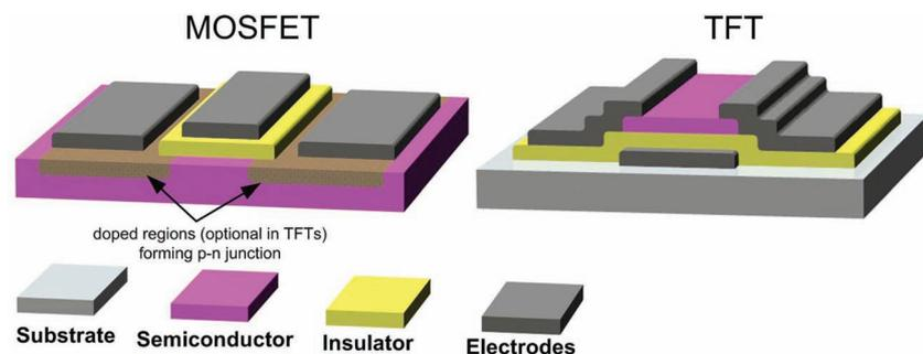
**Figure 8.** Comparison between the typical structures of MOSFETs and TFTs.
