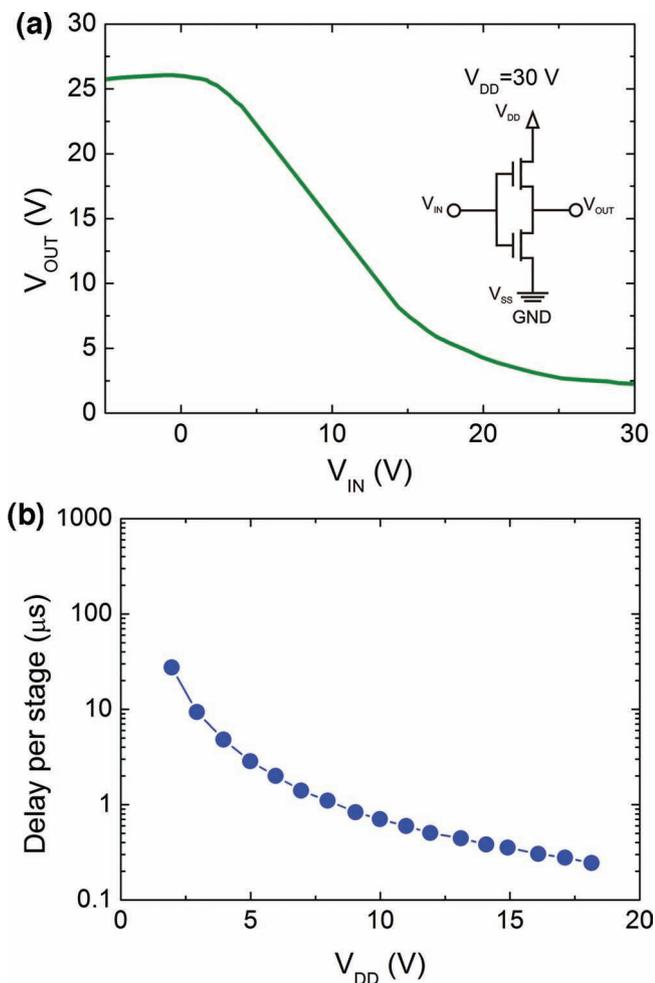
**Figure 53.** Electrical properties of initial oxide TFT based circuits: a) VTC for a transparent inverter using IGO TFTs (adapted from [491]); b) Propagation delay in a RO based on GIZO TFTs (adapted from [225]).
